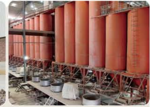
A batch storage system which can reserve 12,000 tons of prepared clay material
