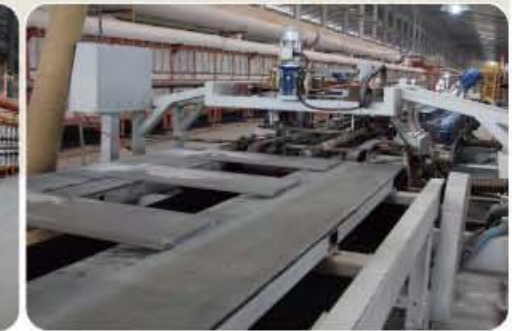
The automatic production line with the processing capacity of shaping, cutting and polishing
